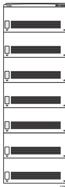
Figure 6 CIX 670 Base/Expansion Cabinets
